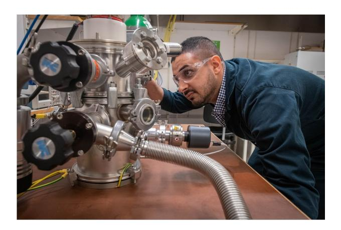
Hama Nadhom adjusts the gas supply to the vacuum chamber in which LiU researchers study how plasma electrons can be used to create thin metallic films. Credit: Magnus Johansson/Linköping University
