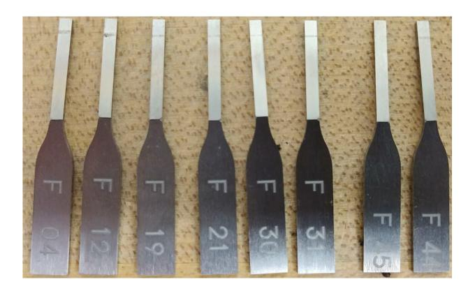
Small samples of titanium alloys were subjected to an intense proton beam at Brookhaven National Laboratory, after which they were tested for stress fatigue at Fermilab. Credit: Sujit Bidhar
