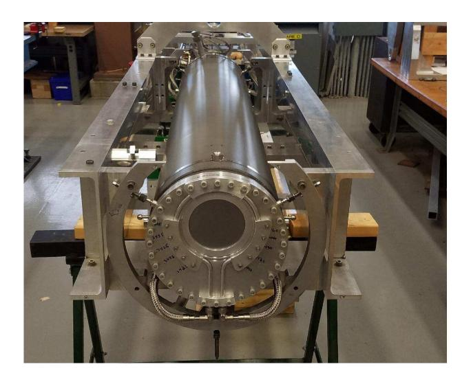
To create neutrinos, a beam of particles smashes into a target, which is contained in a chamber. The beam enters and exits the chamber (seen here on a carrier frame) through highly resilient metallic windows (the dark disk at the front of the chamber), which must be able to withstand a pummeling from the high-
