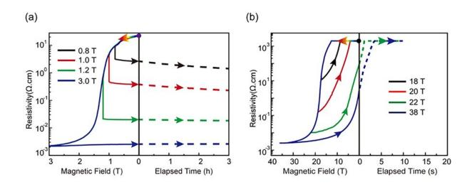
Low-temperature magnetoresistance after zero-field cooling. (a) Magnetoresistance of the alloy film at 10 K after zero-field cooling. (b) Same process as in A but for the ordered film at 0.38 K. Credit: MIAO Tian
