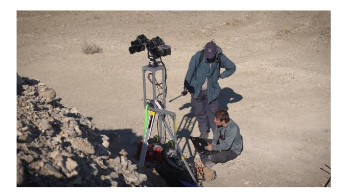
Two members of the field team set up cameras as part of the simulated rover operation. The images they provided were intended to stand in for what a rover's instruments might send back from Mars. Credit: NASA/JPL-Caltech
