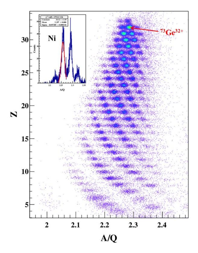
Fig.1. Z versus A/Q particle identification plot for fragments produced in the
