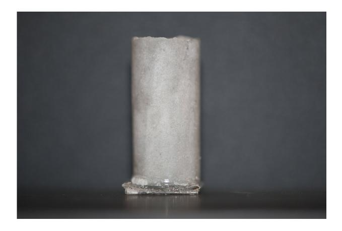
This image shows how concrete with biomimetic antifreeze polymer shows no signs of spalling after 30 freeze-thaw cycles Credit: Living Materials Laboratory, University of Colorado Boulder
