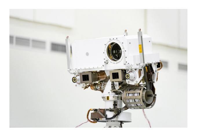
A close-up of the head of Perseverance Rover's remote sensing mast. The mast head contains the SuperCam instrument (its lens is in the large circular opening). In the gray boxes beneath mast head are the two Mastcam-Z imagers. On the exterior sides of those imagers are the rover's two navigation cameras. Credit: NASA/JPL-Caltech
