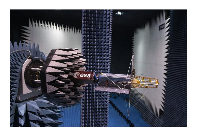
The HiberThree CubeSat underwent antenna testing at ESA's Hertz facility during May 2020. Credit: ESA-P de Maagt
