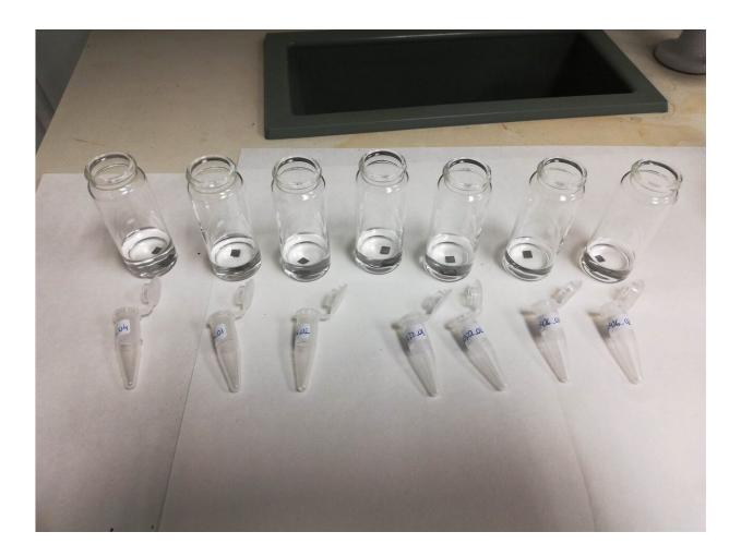
Samples of FeRh metamagnetic material, ready to be analised at the ALBA Synchrotron. Credit: ICMAB-CSIC
