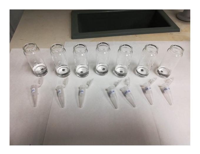
Samples of FeRh metamagnetic material, ready to be analised at the ALBA Synchrotron. Credit: ICMAB-CSIC
