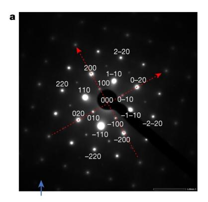
Transmission electron microscopy. a, b, Selected-area electron diffraction pattern obtained from SrTiO3:Al loaded with Rh (0.1 wt%)/Cr2O3 (0.05 wt%)/CoOOH (0.05 wt%) (a) and corresponding transmission electron microscopy image of a particle (b). c, Particle morphology and crystal orientation. Credit: *Nature* (2020). DOI: 10.1038/s41586-020-2278-9
