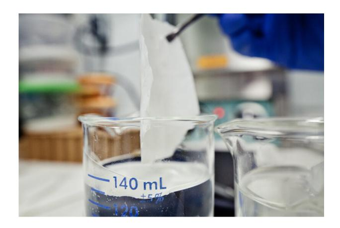
The material consists of Nafion with embedded nanoparticles. Credit: B.Matos/IPEN
