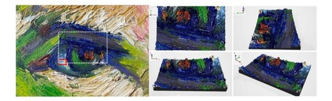
The researchers acquired OCT imaging data of an impressionist-style oil painting (left image). OCT images within the dotted line were digitally stitched together to produce the 3D images shown in the panels on the right. Credit: Yi Yang, Penn State Abington
