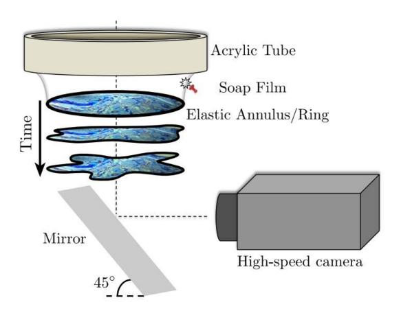
General principle of the experiment: a closed elastic object (a ring or annulus) is held within a soap film. At t = 0, the outer soap film is broken allowing the object, with inner soap film intact, to fall freely. The unbalanced surface tension force from the inner soap film causes the object to buckle dynamically; this motion is captured by a high speed camera. Credit: arXiv:1812.11009 [condmat.soft]
