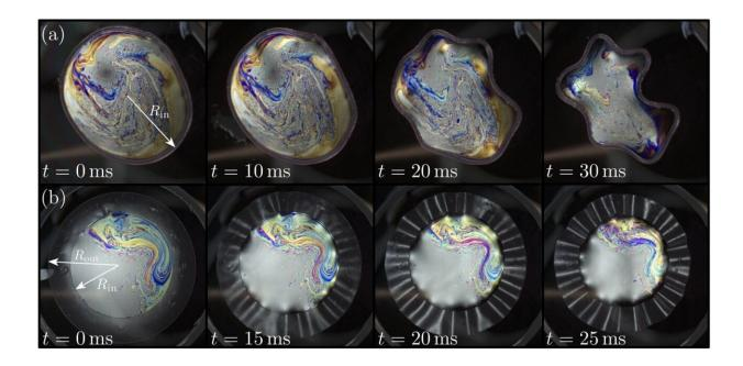
Experimental snap-shots from the dynamic buckling of an elastic (a) ring (h = 1 mm =  $R_{out} - R_{in}$ ,  $R_{in} = 23.5$  mm, E = 42 kPa) and (b) annulus (h = 110  $\mu$ m,  $R_{in} = 25$  mm,  $R_{out} = 34$  mm, E = 200 kPa) under the action of an unbalanced surface tension  $T_{in}$ . Credit: arXiv:1812.11009 [cond-mat.soft]
