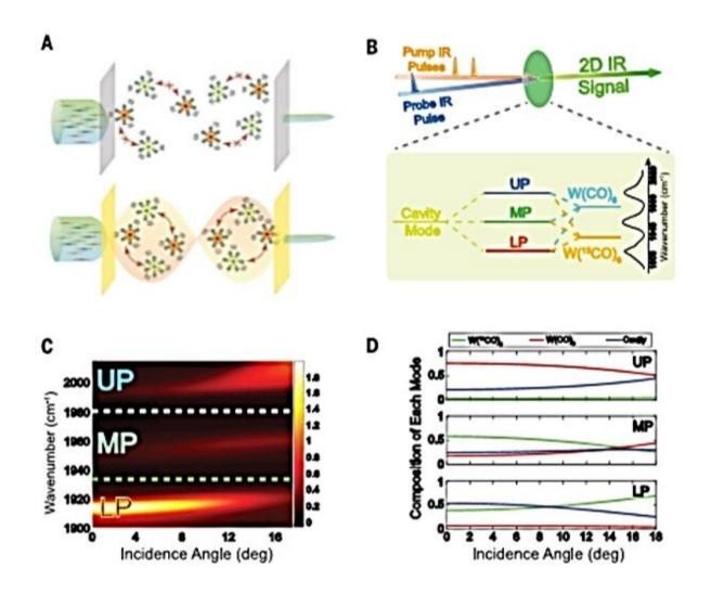
Strongly coupled system between W(CO)6 and W(13CO)6 in a hexane/DCM mixture and a cavity. (A) Schematic illustration showing that VET between vibrational modes of W(CO)6 and W(13CO)6 molecules is unfavorable in solution (top) but is enabled by strong coupling of the molecular system to an
