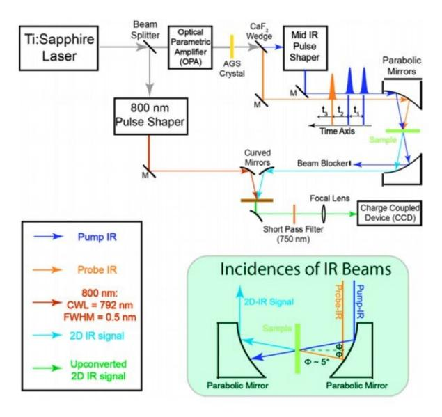
Scheme of two-dimensional infrared experimental setup. The inset shows the incidence of pump and probe IR beams. Credit: Science, doi: 10.1126/science.aba3544
