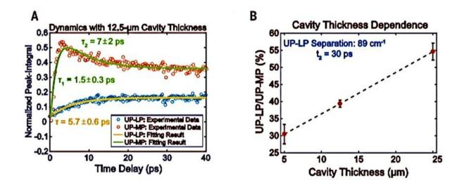
Dynamics and cavity-thickness dependence of polariton-enabled intermolecular VET. (A) Dynamics of [wUP, wLP] and [wUP, wUP] peak integrals and the fitting results. The sample was taken at an incidence angle of 15°. (B) Plot of IUP,MP/IUP,LP as a function of cavity thickness at t2 = 30 ps. Error bars represent the SD of three independent scans. Credit: Science, doi: 10.1126/science.aba3544
