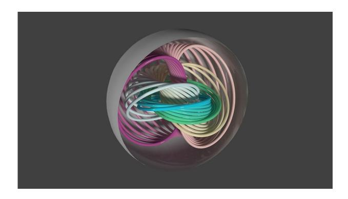
Image depicts some of the polarization lines within a ferroelectric nanoparticle. The lines intertwine into a Hopfion topological structure. Credit: Image by Yuri Tikhonov, University of Picardie and Russia's Southern Federal University, and Anna Razumnaya, Southern Federal University
