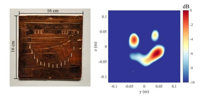
A smiley-face-shaped antenna (left) is correctly identified by a new method for passively locating radio wave sources (right). Credit: Aaron Diebold, Duke University
