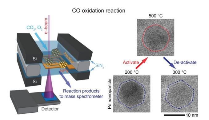
Figure (left) shows the setup used in the capturing of reversible transformations in Palladium (Pd) nanoparticles during carbon monoxide (CO) oxidation reaction with operando transmission electron microscopy (TEM). These transformations determine the catalytic activity of the nanoparticles. (Right) TEM images of Pd nanoparticles under different temperature conditions. Credit: Nature Communications
