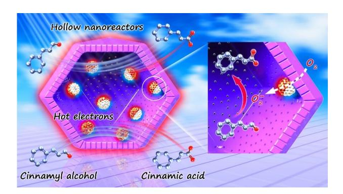
Schematic diagram of hollow nanoreactors for photocatalytic oxidation of cinnamyl alcohol. Credit: Science China Press
