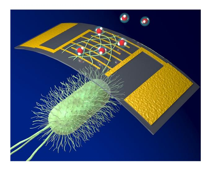
Protein nanowires (light green) harvested from Geobacter (background) are sandwiched between electrodes (gold) to form bioelectronic sensor for detection of biomolecules (red). Credit: UMass Amherst/Yao lab
