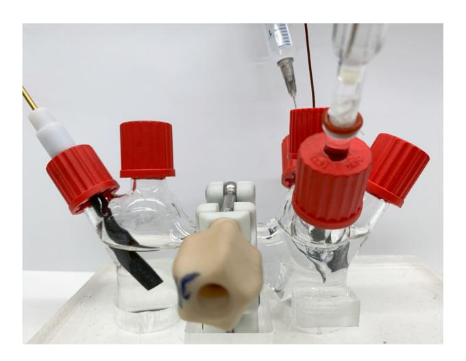
The researchers' H-cell setup for developing their hydrogen peroxide production method. Credit: University of California - San Diego
