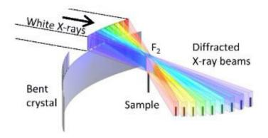
How the bent crystal changes the direction of the x-rays. Credit: Tohoku University
