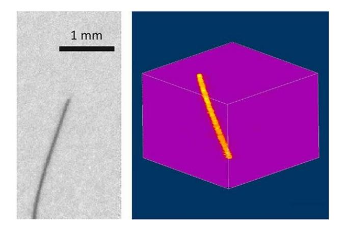
On the left is a projection image obtained with an exposure time of 1 ms whilst on the right is a three-dimensional reconstruction obtained from 32 projection
