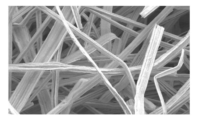
An electron microscope view of the nickel felt material that optimized surface area and bubble release as it produced hydrogen from electrolysis. Credit: Wiley Lab, Duke University
