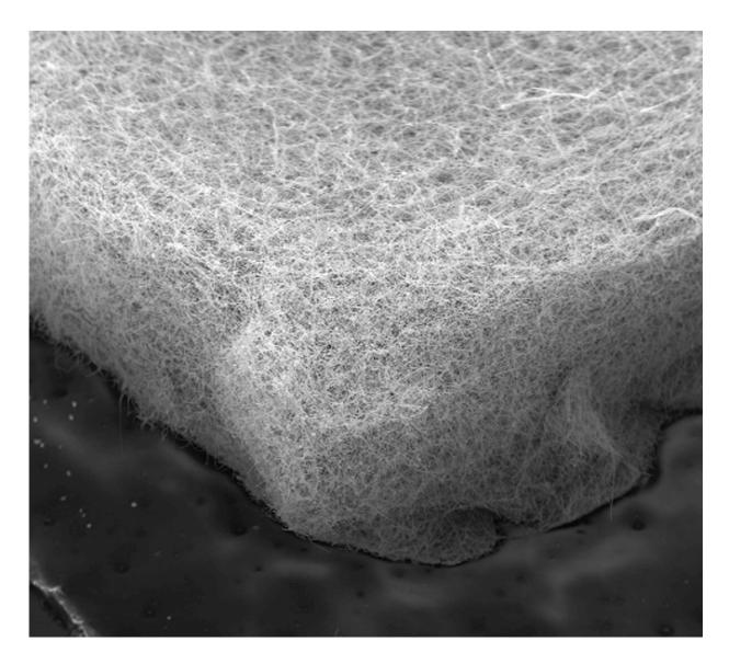
A microscopic view of the nickel felt material thatoptimized surface area and bubble release as it produced hydrogen from electrolysis. Credit: Wiley Lab, Duke University
