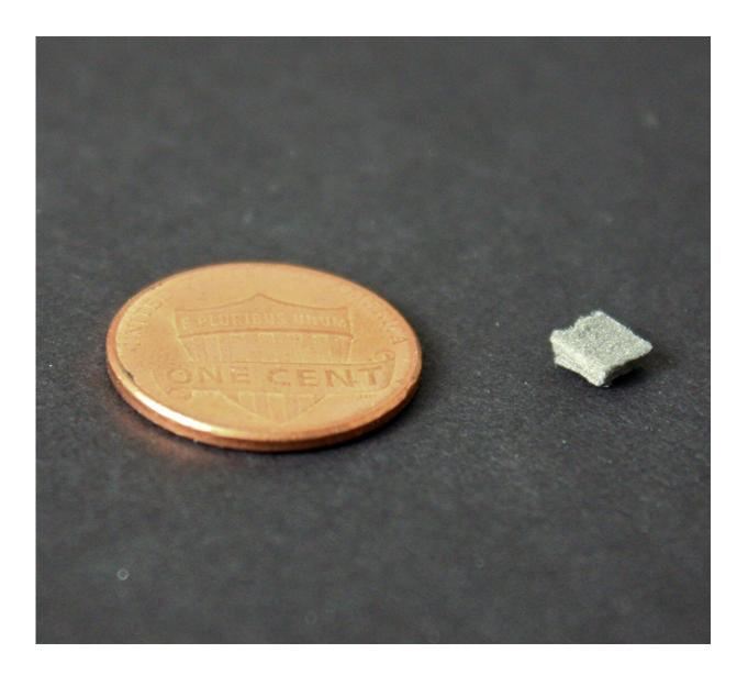
An example of the small, flow-through electrode that Duke researchers used to produce more hydrogen from electrolysis with a penny for scale. Credit: Wiley
