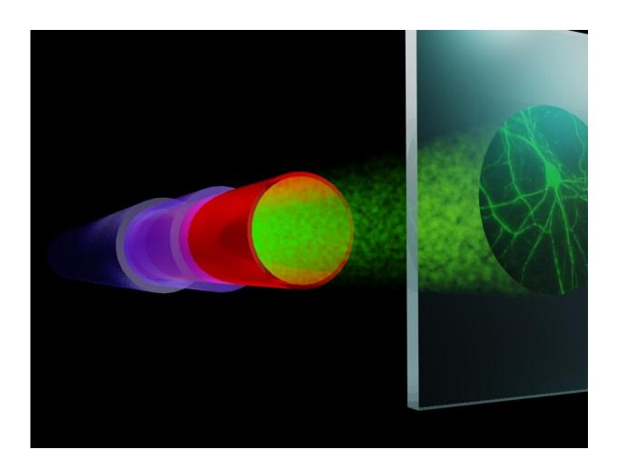
Artist impression of the super-resolution fiber setup. A randomly speckled beam (green) from the fiber illuminates the entire sample (right) several times. Compressive sensing reconstruction offers a high-resolution image of the sample without the need for fluorescent labeling, offering nanoscopy applications in both bioimaging and nanolithography. Credits: Lyuba Amitonova
