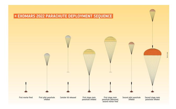
The ExoMars parachute deployment sequence that will deliver a surface platform and rover to the surface of Mars in 2021 (following launch in 2020). The graphic is not to scale, and the colours of the parachutes are for illustrative purposes only. Credit: European Space Agency
