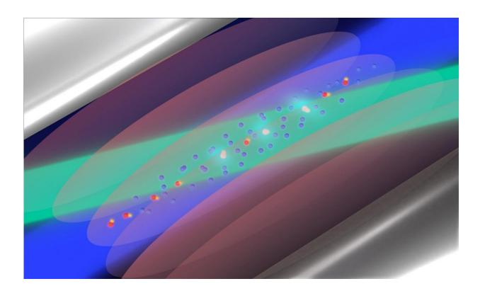
HD+ molecular ions (yellow and red pairs of dots: proton and deuteron; the electron is not shown) suspended in an ultra-high vacuum between atomic ions (blue dots), which are immobilised using a laser beam (blue). An electromagnetic wave (red-brown discs) causes the molecular ions to rotate. A further laser beam (green) records evidence of this excitation. The drawing is not to scale. Credit: HHU / Alighanbari, Hansen, Schiller
