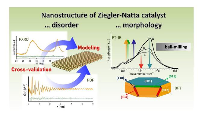
The nanostructure of the heterogeneous Ziegler-Natta catalyst was clarified on the basis of cutting-edge analytical techniques. Left: Typical synchrotron data and the determined nanoparticle model of the catalyst primary particle. Right: Experimental Far-IR spectra of a series of catalyst supports, and Wulff's polyhedra derived on the basis of surface formation energy. Credit: Japan Advanced Institute of Science and Technology
