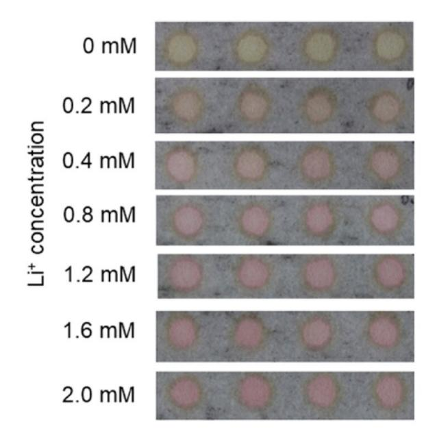
The colorimetric detection unit displays diagnostic colors depending on the concentration of lithium ion. F28 tetraphenylporphyrin is used for the detection reagent. Credit: Komatsu T. et al., ACS Sensors, April 23, 2020
