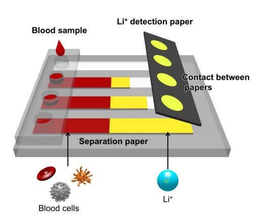
The newly developed paper-based device can easily and cheaply measure lithium ion concentration in blood. Credit: Komatsu T. et al., ACS Sensors, April 23, 2020
