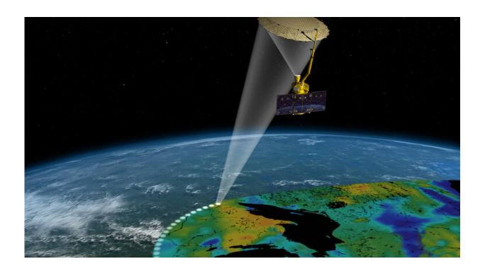
Artist's rendering of the Soil Moisture Active Passive satellite. The width of the region scanned on Earth's surface during each orbit is about 620 miles. Credit: NASA/JPL-Caltech
