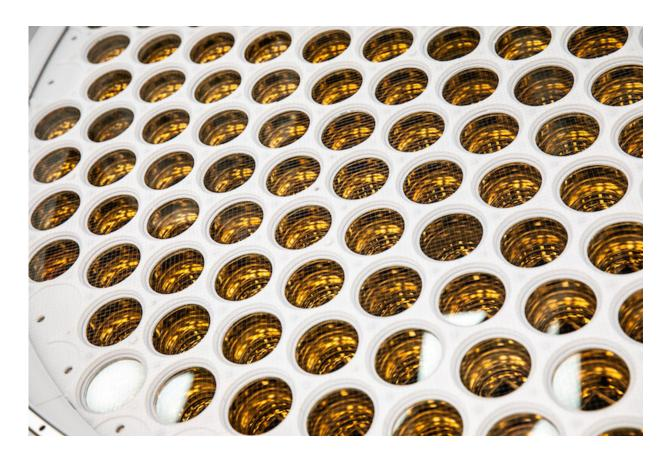
Photomultiplier tube arrays are prepared for the WIMP-hunting LUX-ZEPLIN experiment during assembly at the Sanford Underground Research Facility in Lead, South Dakota. Credit: Matt Kapust/SURF
