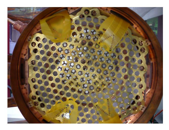
The EXO-200 time projection chamber during assembly. Credit: EXO-200 collaboration
