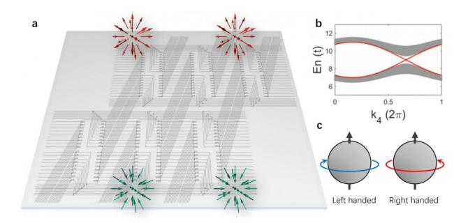
(a) The 4D circuit lattice realized on a 2D plane. A pair of Weyl points with the same chirality are localized on the three-dimensional boundary. (b) The bulk band structures and the boundary Weyl states (red lines). (c) Schematic of the chirality of Weyl states. Credit: Science China Press
