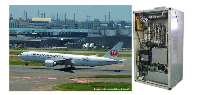
(left) Japan Airlines aircraft with a special project logo (CONTRAIL) taking off at Tokyo International Airport and (right) Continuous CO<sub>2</sub> Measuring Equipment onboard the aircraft Credit: CONTRAIL Team (Japan Airlines)
