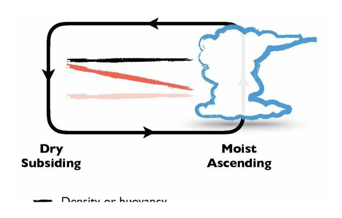
This graphic illustrates the vapor buoyancy effect, in which cold, humid air rises because it is lighter than dry air. Credit: Da Yang/UC Davis
