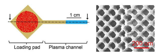
The layout of the filter and a close-up of the surface detail. Clotted blood cells are indicated in red. Plasma filling up the channel is indicated in yellow. And the blue section indicates the empty remainder of the channel as the plasma fills it in. Credit: KTH Royal Institute of Technology
