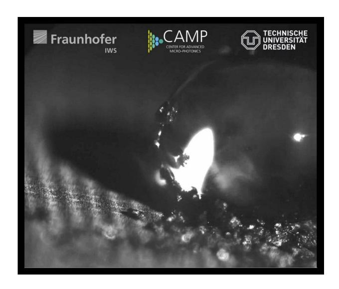
Water drops do not adhere to the self-cleaning aluminium surface. The latter has been functionalized by a team of CAMP scientists using direct laser interference
