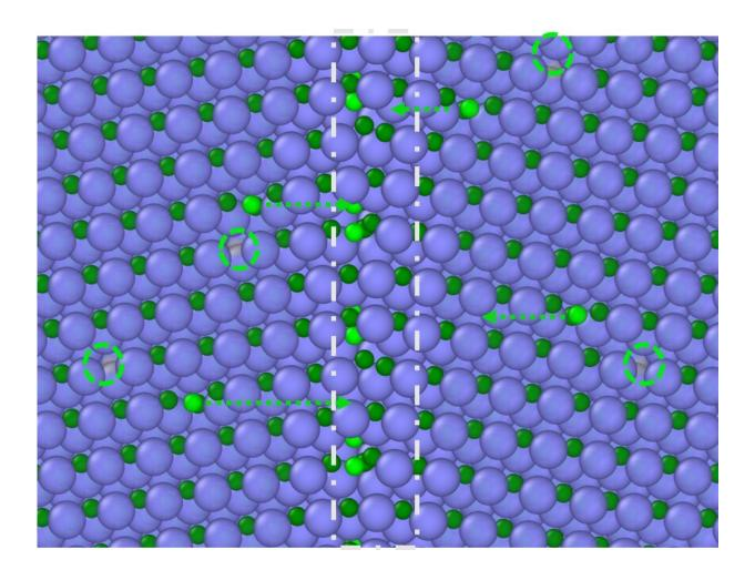
Silicon carbide after irradiation, in which loose carbon atoms (green) move toward the boundary (dashed line) between grains of the crystalline ceramic. Credit: Hongliang Zhang
