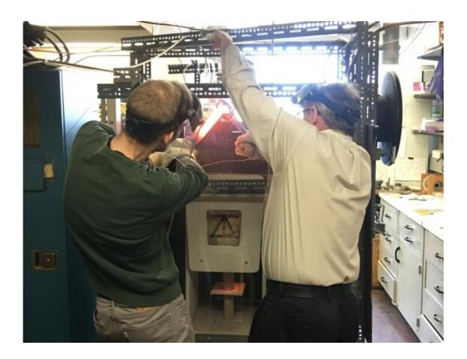
Max Collinet PhD '19 (left) and Professor Tim Grove work together to extract an experimental sample from a one-of-a-kind rock-melting machine at MIT that reveals clues about planetesimals and the formation of the rocky planets like Earth and Mars. Credit: Stephanie Brown/MIT
