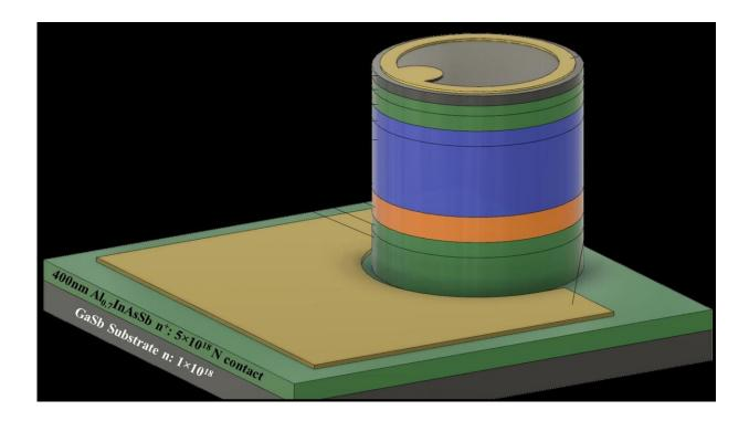
Epitaxial cross section of the avalanche photodiode design. Doping concentrations are given in cm<sup>-3</sup> Credit: Joe C. Campbell
