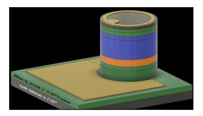
Epitaxial cross section of the avalanche photodiode design. Doping concentrations are given in cm<sup>-3</sup> Credit: Joe C. Campbell
