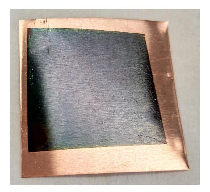
The new catalyst is an alloy of copper and aluminium with a unique nanoscale porous structure. Credit: Alexander Ip / University of Toronto Engineering
