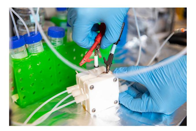
Researchers from U of T Engineering and Carnegie Mellon University are using electrolyzers like this one to convert waste CO2 into commercially valuable chemicals. Their latest catalyst, designed in part through the use of AI, is the most efficient in its class. Credit: Daria Perevezentsev / University of Toronto Engineering
