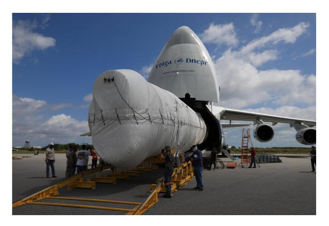
The first stage of the United Launch Alliance Atlas V that will carry NASA's Perseverance rover into space is offloaded from an Antonov cargo plane at Kennedy Space Center in Florida on May 11, 2020. Credit: NASA
