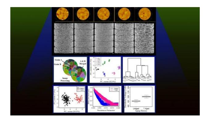
Topological analysis of X-ray CT data for recognition and trending of changes in microstructure under material aging. Credit: Lawrence Livermore National Laboratory
