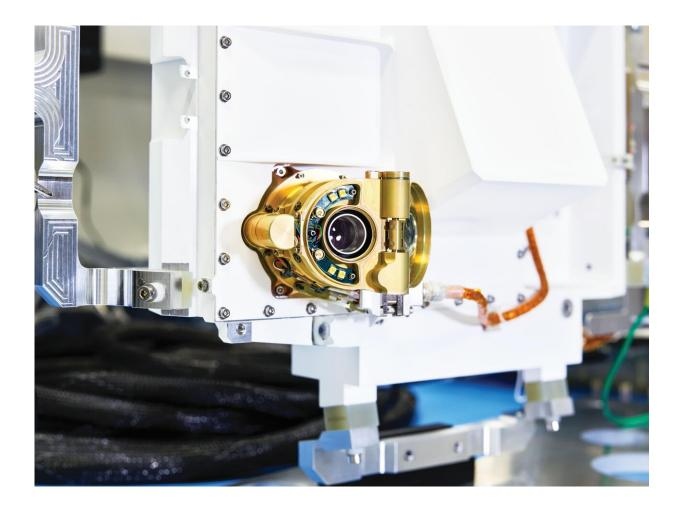
An engineering model of SHERLOC, one the instruments onboard NASA's Perseverance Mars rover. Located on the end of the rover's robotic arm, SHERLOC will help determine which samples to take so that they can be sealed
