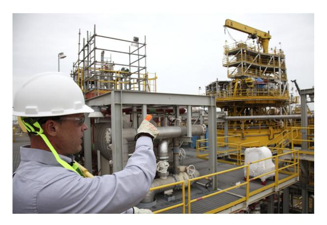
In this Tuesday March 10, 2020 photo, David Nickerson, CEO of Marine Well Containment Company, points to the hydrocarbon train that fits on top a oil spill disaster response tanker, in Ingleside, Texas. The device helps process spilled oil and other hydrocarbons. It also helps collect oil spewing out of blown out deep sea wells for storage in oil tankers hulls.(AP Photo/John L. Mone)
