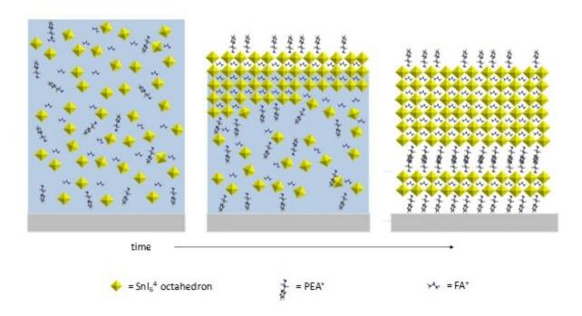
The scheme of the mechanism of crystallization from DMF/DMSO solution during drying for the 2D/3D perovskite films. Credit: G. Portale, University of Groningen
