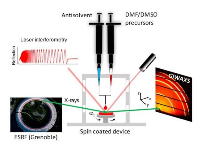
A scheme of the experimental setup used to investigate the structural formation of perovskites thin films during spin coating. Credit: G. Portale, University of Groningen
