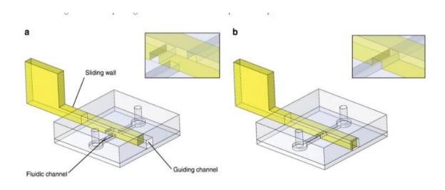
Sliding wall principle. PDMS structures contain a guiding channel and a fluidic channel and were bonded to a planar PDMS surface. In this example, a sliding wall with an engraved channel was inserted after chip fabrication inside the guiding channel. The fluidic channel was a blocked or b free. Details of the sliding wall/fluidic channel intersection are provided in the inserts. Credit: Microsystems & Nanoengineering, doi: 10.1038/s41378-019-0125-7
