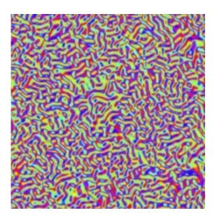
Disordered pattern of eddies of a characteristic size. The color code indicates the local orientation of the liquid crystal. Credit: University of Barcelona
