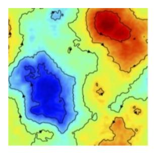
Large-scale circulating flows at scales much larges the the characteristic size of the underlying pattern of vortices. Credit: University of Barcelona
