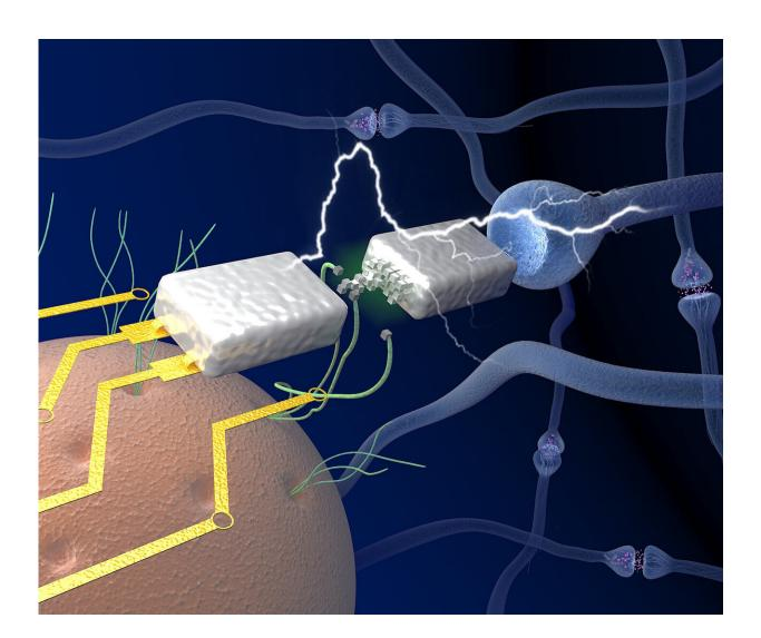
A graphic depiction of protein nanowires (green) harvested from microbe Geobacter (orange) facilitate the electronic memristor device (silver) to function with biological voltages, emulating the neuronal components (blue junctions) in a brain. Credit: UMass Amherst/Yao lab
