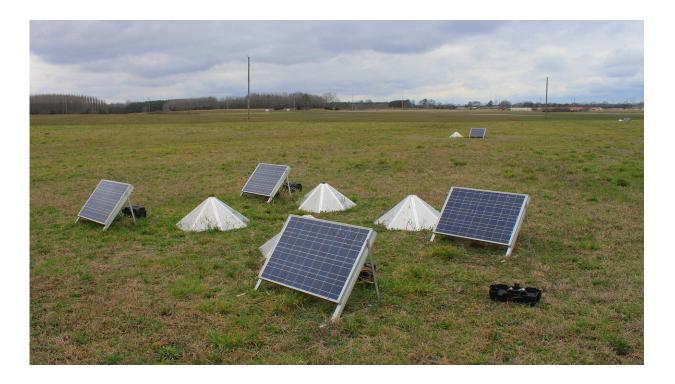
Infrasound array sensors accurately record infrasonic signals as part of research by the UM National Center for Physical Acoustics into tornado detection and tracking. Credit: Shea Stewart/University of Mississippi
