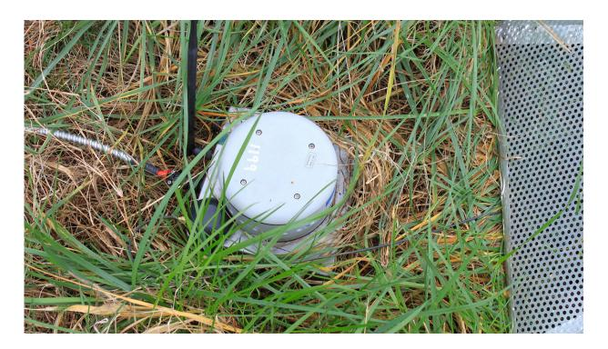
Sensors designed at UM record infrasonic signals, acoustic signals at frequencies below what humans can hear. Credit: Shea Stewart/University of Mississippi
