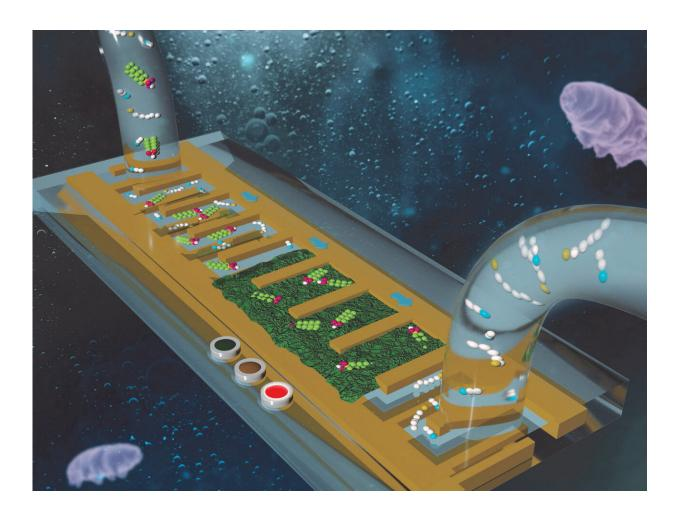
An illustration of PNNL's PFAS Sensor. Water samples flow in one end, through the maze and PFOS gets captured by a sponge-like material in the middle. The technology is available for licensing. Credit: Nathan Johnson | PNNL
