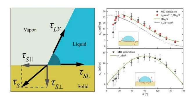
Theoretical model and verification of capillary force balance at the three-phase contact line. Credit: FAN Jingcun et al.
