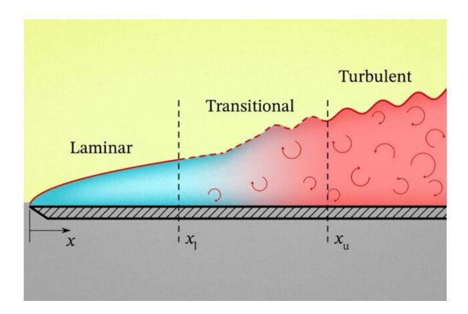
Fluids that heat or cool surfaces make a transition from a smooth flow to a mixing, turbulent flow. A new MIT analysis shows the importance of the transition region to heat flow and temperature control. Credit: Courtesy of the researchers, edited by MIT News
